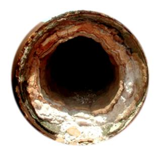
Scales are inorganic mineral components of water. Hence, the key concept in scaling is solubility. Solids may precipitate as they (ions) have low solubility in water and deposit from the brine once the solubility limit or capacity has been reached.
